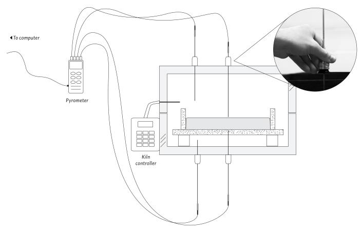
Figure 1: A multi-point monitoring system
