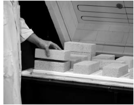
Figure 11: weighting the fiberboard shelf with bricks.
