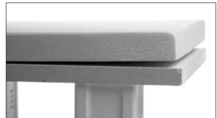
Figure 12: example of a bowed fiberboard shelf corner.
