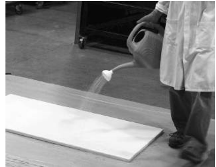
Figure 6: a watering can with a showerhead spout will control the flow of colloidal silica.
