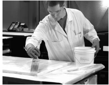
Figure 8: Brushing qf-180 onto the fiberboard shelf.
