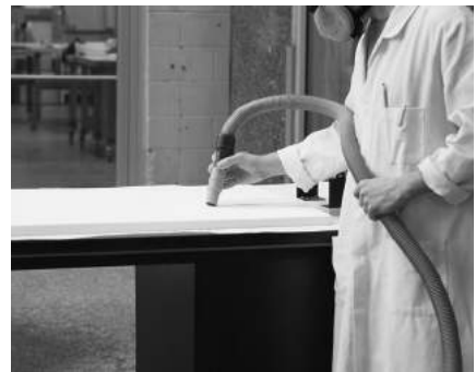
Figure 10: vacuuming dust from the shelf after sanding.
