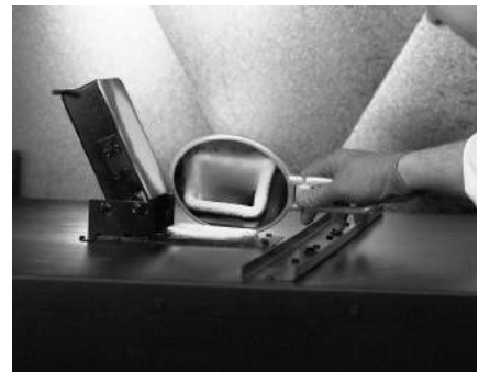
Figure 7: using a mirror to check for condensation.
