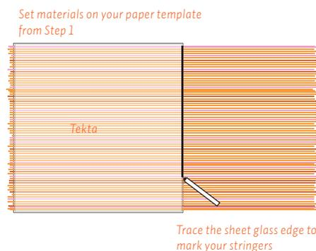
Note: If using stringers that already have one nicely cut end, set the "clean" ends flush with one side of the template instead of cutting them.
