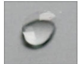
Remember - A ball means TIN. So fire this side **DOWN** to minimise any tin effects
